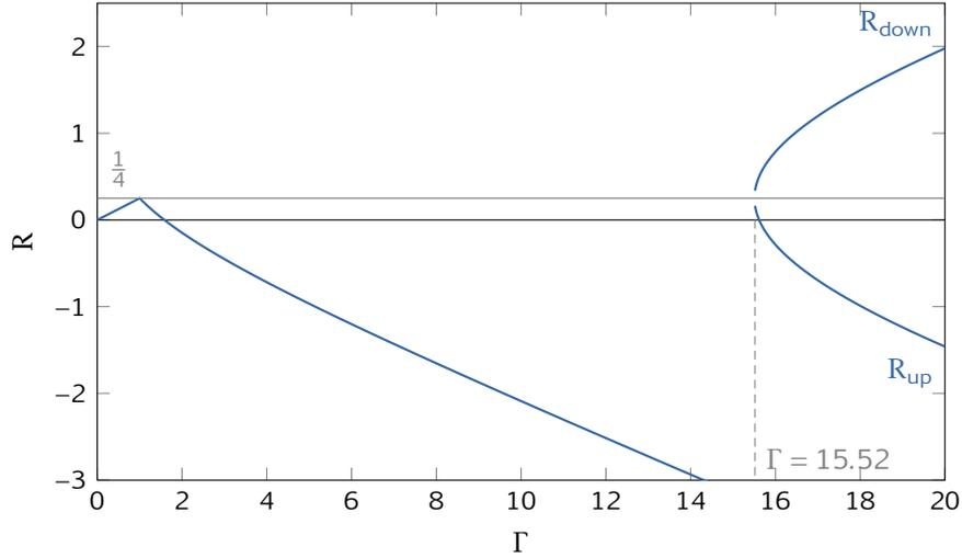
Figure 4: Variations of the function  $R$  expressed in (51). This function is inferior to  $1/4$  for the primary branch of nontrivial solutions (starting at  $\Gamma = 1$ ). For the secondary branch (starting at  $\Gamma = 15.52$ ), one solution is stable ( $R < 1/4$ ) while the other one is unstable ( $R > 1/4$ ).
