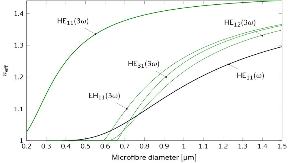
Figure 3: Evolution of the effective indices of the different modes of interest in a silica microfibre according to the microfibre diameter. The wavelengths are 1550 nm (pump, black curve) and 517 nm (third-harmonic, green curves). Phase-matching condition is fulfilled at any intersection of the black curve with one of the green curve.
