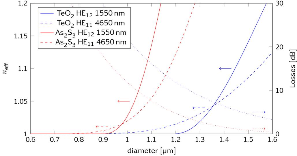
Figure 7: Index variation of the  $HE_{11}$  (4650 nm) and  $HE_{12}$  (1550 nm) modes in tellurite and chalcogenide as a function of the diameter of the microfiber. Phase-matching diameters for triple photon generation are  $1.36 \mu\text{m}$  in tellurite fibers and  $980 \text{ nm}$  in chalcogenide fibers. Losses, calculated for a characteristic taper transition length  $L=100 \mu\text{m}$ , are represented with dotted lines and on the right  $y$ -axis.
