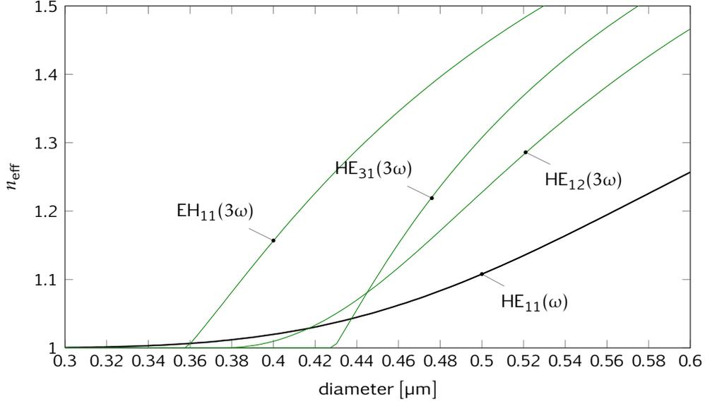
Figure 5: Effective indices of modes in a 20Na<sub>2</sub>O tellurite glass at both pump (1560 nm) and TH (520 nm) wavelengths.
