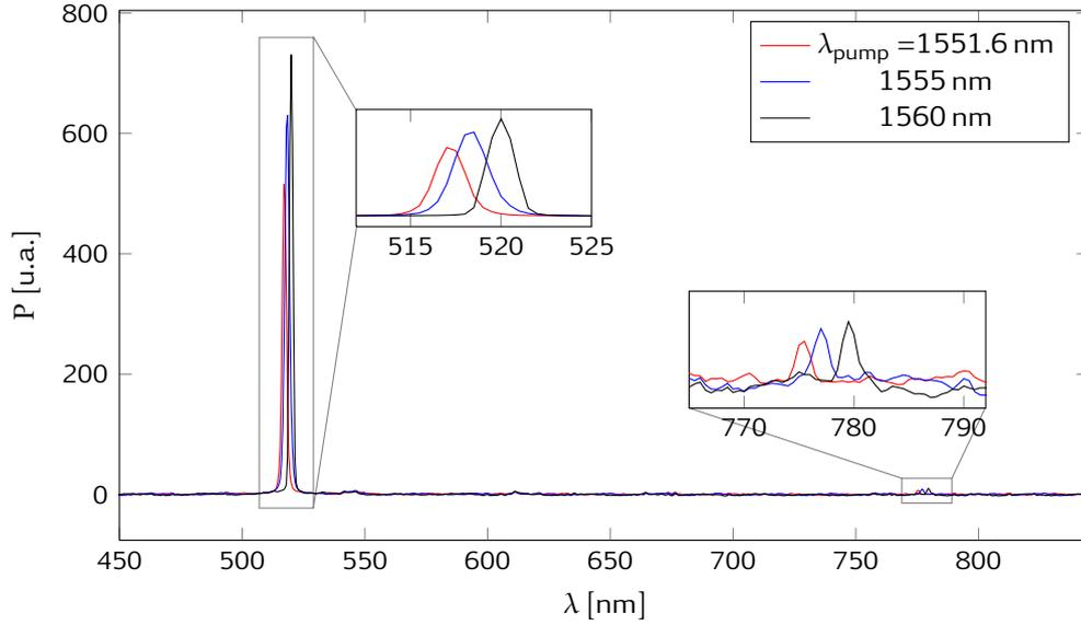
Figure 1: Spectrum of the third-harmonic wave, generated around 520 nm by pumping the same microfibre at three different wavelengths. A small amount of second-harmonic wave around 780 nm is also visible, see its magnification.
