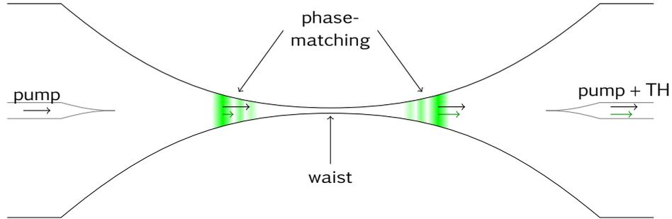
Figure 4: Phase-matched THG occurs in the taper transitions, allowing for broadband conversion
