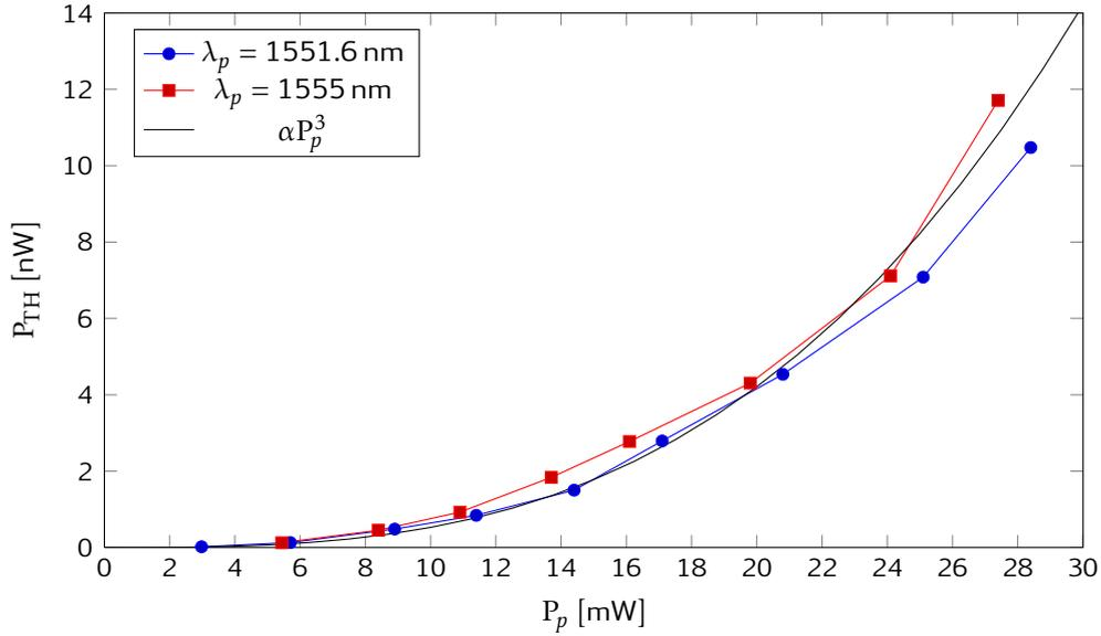
Figure 2: Evolution of the converted THG power as a function of the pump power for two different pump wavelengths. A cubic curve is also plotted for comparison. All powers are measured after propagation in the microfibre.
