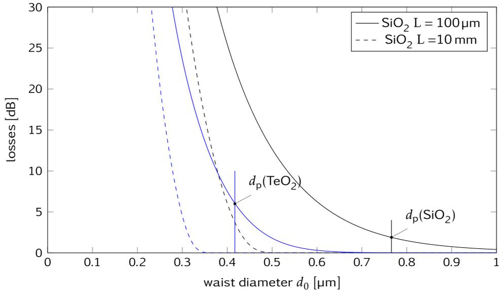
Figure 6: Evaluation of fundamental radiative losses in microfibres at the pump wavelength (1550 nm) using the theory of nonadiabatic intermode transitions. Silica and tellurite microfibres are studied for different characteristic lengths  $L$  of diameter variation.
